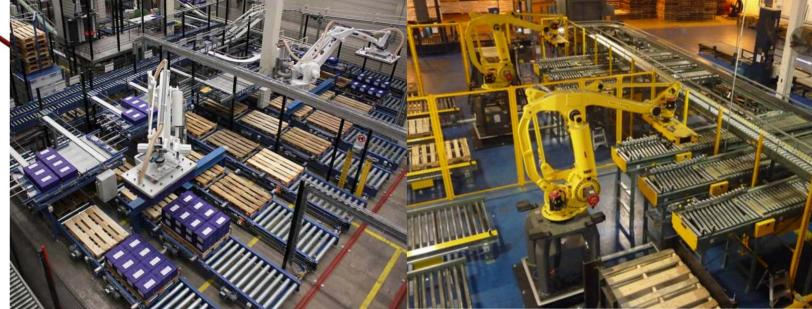
MCS Production technology finalises its lines with completely automatic robotic palletising systems, by using robots with different payload capacities and reaches, which are fed by automatic shuttles for loading and unloading pallets.
